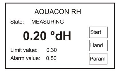
The automatic analysis cycle can be interrupted at any stage by touching the button "Hand" or the button "Param" on the touchscreen (see chapter 3.5).
